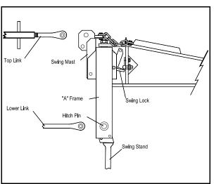
Figure 3. Hitch Adjustment
